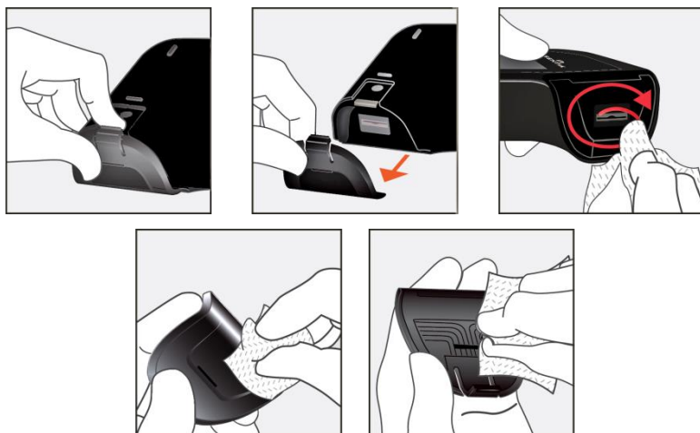
Cleaning spills around the sample port
